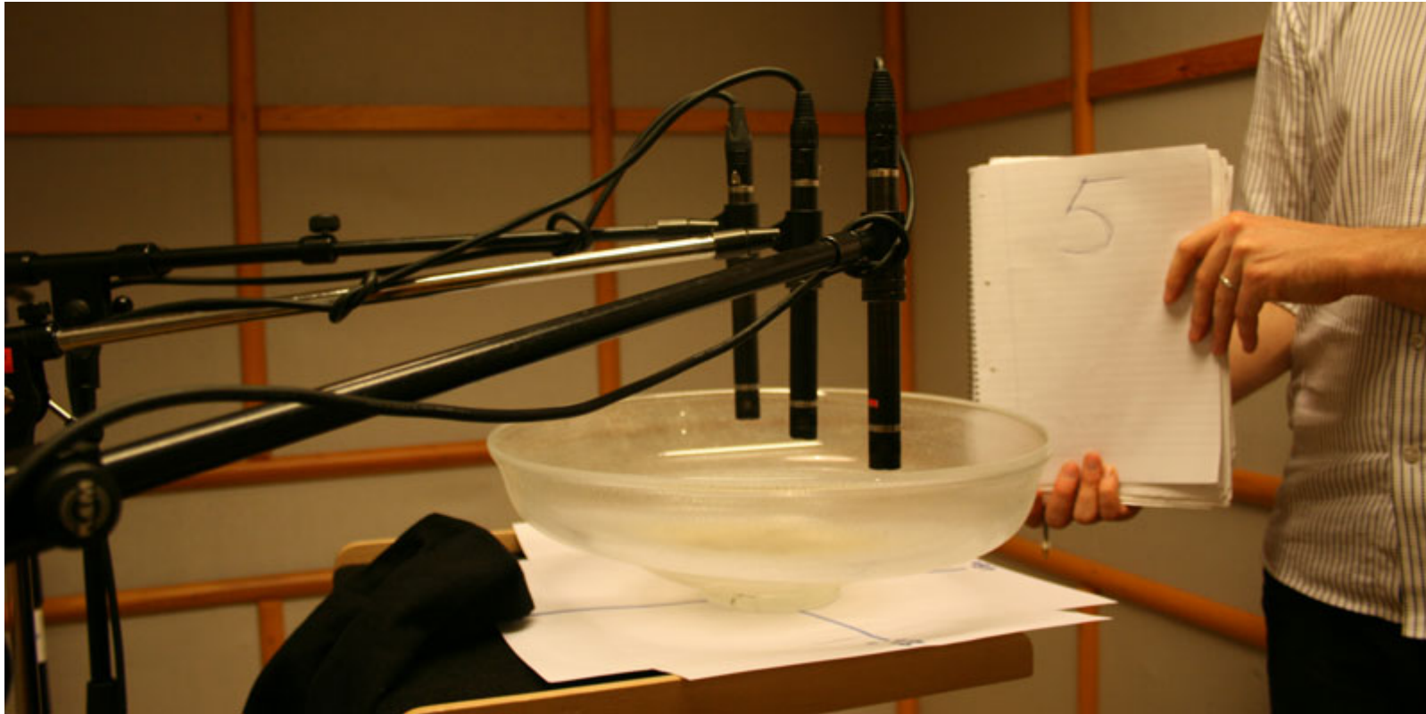
Figure 3: Microphone placement 0.5 cm above the surface, at rim, half-centre and centre positions.
